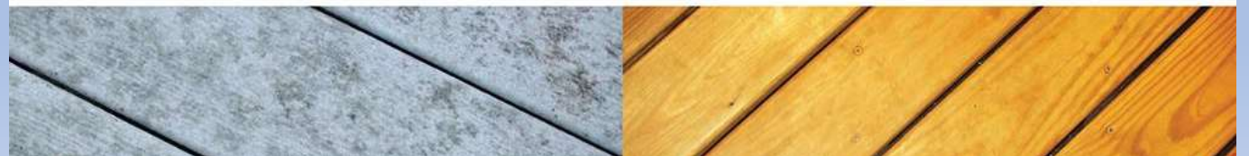
CLEANED AND LEFT UNTREATED Results after 9 months
